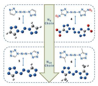
Scheme 2. Synthesis and the optimized structure of 1,1'-azobis-1,2,3triazole (3) and 2,2'-azobis (5-nitrotetrazole) (4) with an  $N_8$  chain, as well as 1,1'-azobis(tetrazole) (5) and 1,1'-azobis(5-methyltetrazole) (6) with an N<sub>10</sub> chain.
